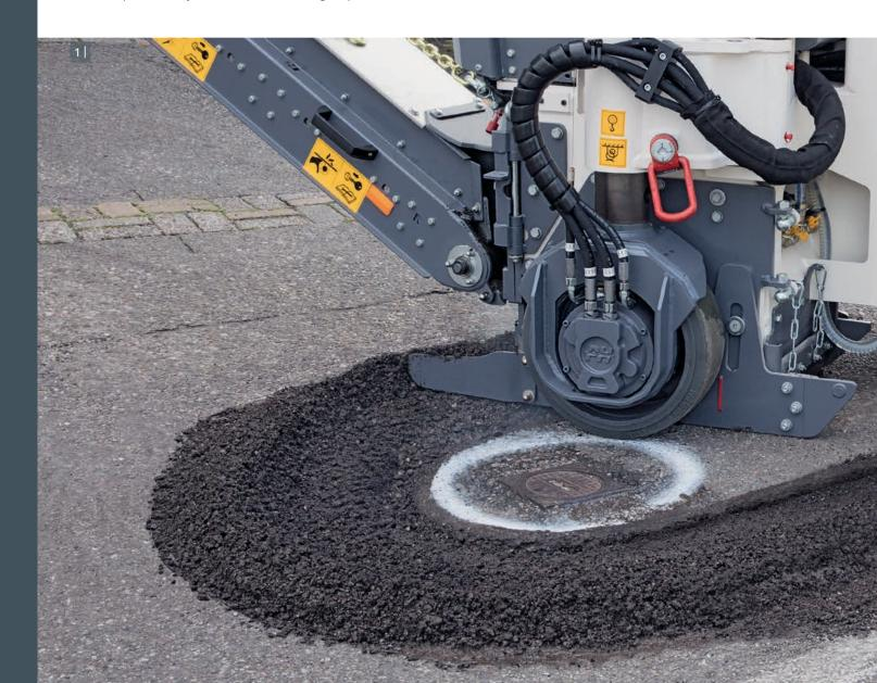
1 - 2 | Electronic traction drive control enables precise milling along road fixtures for example.
