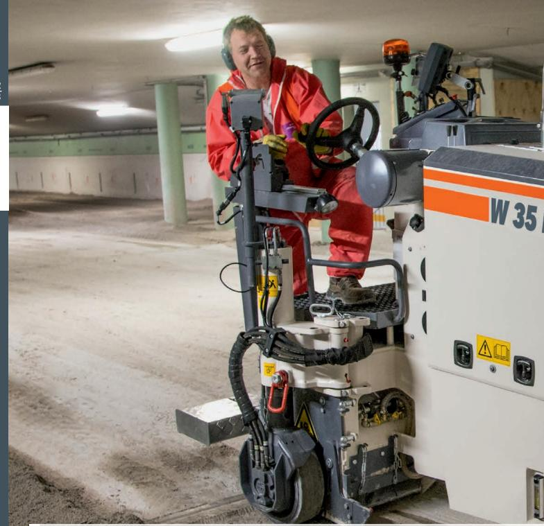
THE MANEUVERABLE COLD MILLING MACHINE IS THE IDEAL CANDIDATE FOR MILLING OPERATIONS IN RESTRICTED SPACE CONDITIONS.
