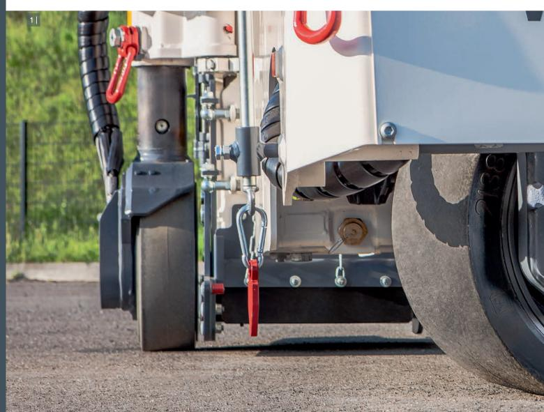
2 Quick maneuvering in narrow passages is an easy exercise for the small milling machine because the right-hand rear wheel can simply be pivoted in front of the milling drum.
